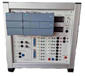
Digital Voltage Display is direct conneted with SUB-D 1 to measure the height of the workpieces, if you connect MCS-520 there, or to show the voltage on the safety plug (Switch).
