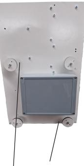
On the backside of the elevator are 4 devices to put the elevator into a DIN A4 frame like as in Electric Labs.
