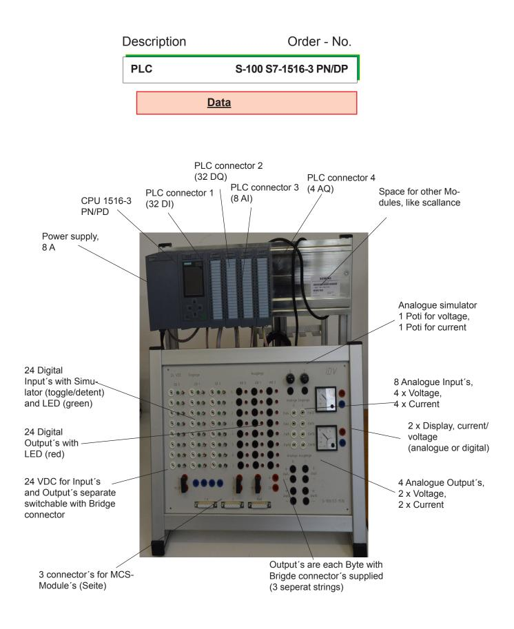
The analog inputs and outputs are wired according to the description above. If you would like to use an input or output as a power input/output, please note the instructions in the SIEMENS manuals.
